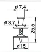
Powder-actuated fastener and fastening tool:
