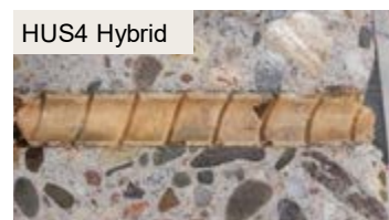
Fig. 3 Thread cut by Hilti HUS4 screw and Hilti HUS4 bonded screw fastener (Hilti HUS4 concrete screw with Hilti HUS4-MAX capsule)
