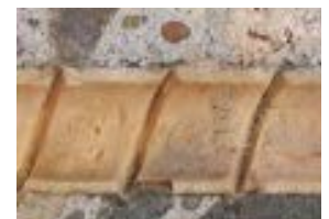
Fig. 3 Thread cut by Hilti HUS4 screw and Hilti HUS4 bonded screw fastener (Hilti HUS4 concrete screw with Hilti HUS4-MAX capsule)
