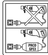
1. Plug the machine's supply cord into an earthed/grounded power outlet.
