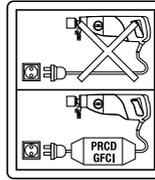
Operate the equipment only with a properly functioning GFCI.
