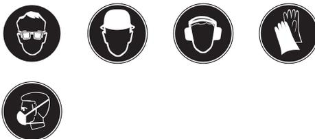
The user and any other persons in the vicinity must wear ANSI Z87.1-approved eye protection, a hard hat, ear protection, protective gloves and breathing protection while the machine is in use.
